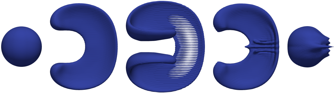
Figure 11: Zero level set \{\phi_h = 0\} representing the surface of the distorted sphere at t = 0, 0.7, 1.5, 2.3 , and 3 . Solutions obtained using linear finite elements with 1, 030, 301 DOFs.
