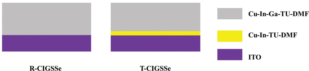
Figure 1. The recipe of CIGSSe absorbers with or without interface treatment.
