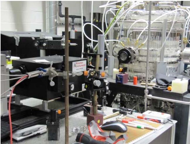
Figure 1: High pressure, high temperature gas flow cell for studying the fluorescence behaviour of fuel tracers using laser-induced fluorescence (LIF)
