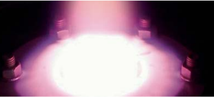
Scale up – nanoparticles for industrial applications Plasma reactor for the synthesis of nanoparticles
