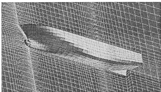
Fig. 2 Discretisation (coarse) and main particulars of RoRo passenger ferry
