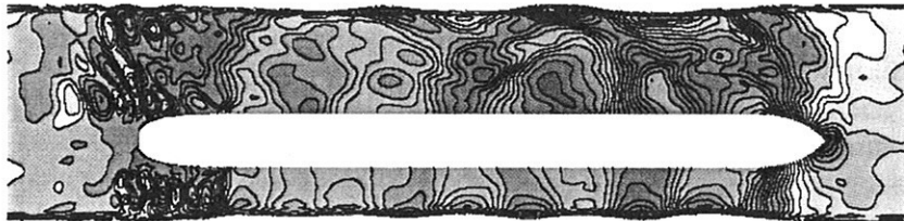
Fig. 2a: Free surface elevation for ship in off-centre position
