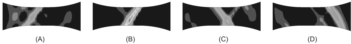
Figure 2: The morphology of simulated PLC bands based on Estrin model.
