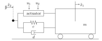
The dynamics of the positioning system shown in the figure should be examined. Regarding only the mechanical part, it can be described by
