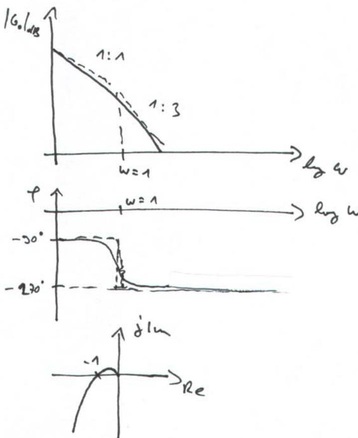
$$\begin{aligned} G(j\omega) &= \frac{1}{j\omega} \frac{1}{-\omega^2 + j\omega + 1} \\ &= \frac{-\omega^2}{\omega^4(\omega - \omega^3)^2} - j \frac{\omega - \omega^3}{\omega^4(\omega - \omega^3)^2} \end{aligned}$$
