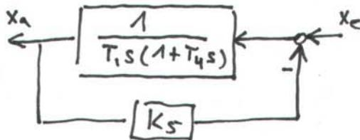
$$(x_e - K_5 x_a) \frac{1}{T_1 s (1 + T_4 s)} = x_a$$
