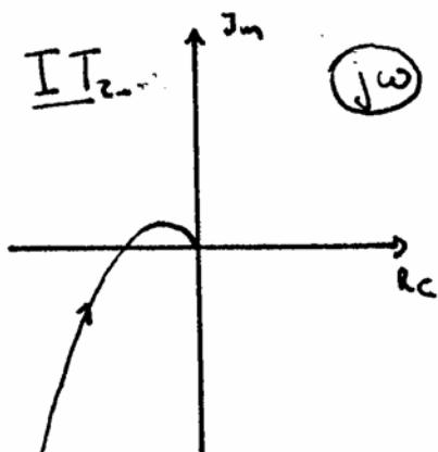
f) - If the crit. point is enclosed, closed-loop system is unstable
