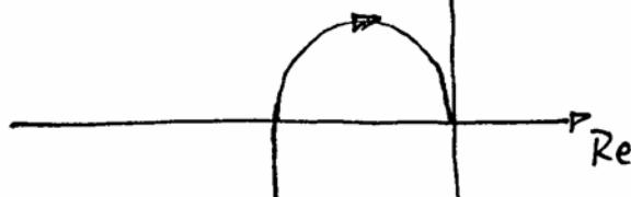
Cf. From the polar plot of the open-loop system and special Nyquist criterion, it can be known that the system is stable, when
