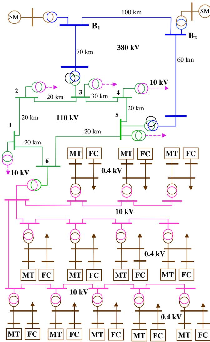
Buses 1 to 5 are extended to the low voltage area with similar integration of Micro-Turbines (MT) and Fuel Cells (FC) like that shown for bus 6
