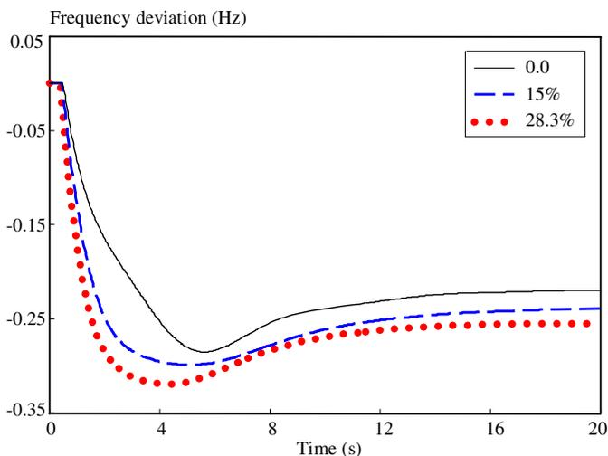
Fig. 7. Frequency deviation as a result of a 10MW (~6% of the total power generation) load switching in the high-voltage network
