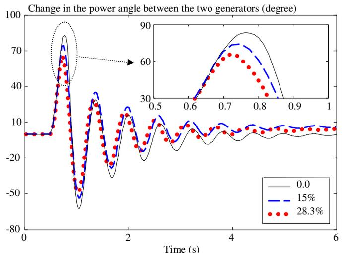
Fig. 6. Variation of the power angle between the two generators due to a fault in the high-voltage network: case 2, some of the DG units are switched off
