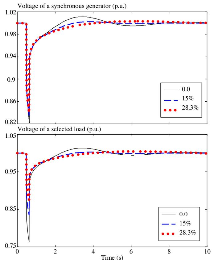
Fig. 8. Voltage variation of one of the synchronous generators and a selected load as a result of a three-phase fault in the high-voltage network
