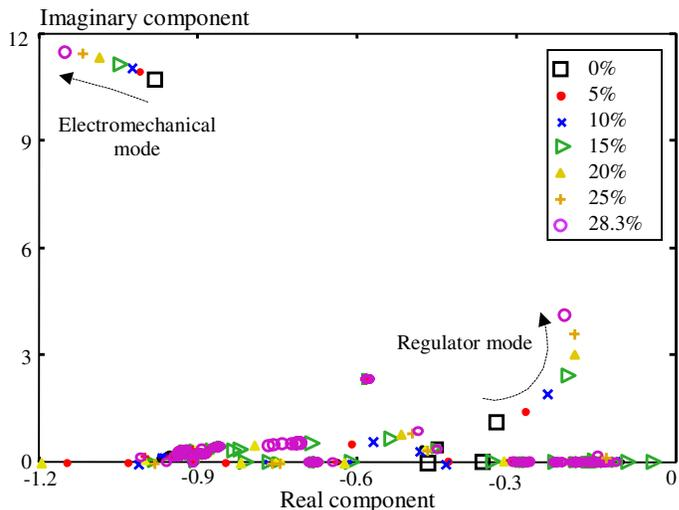
Fig. 4. Critical eigenvalues with different power contributions from DG units
