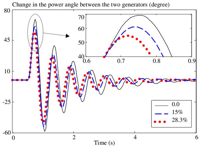
Fig. 5. Variation of the power angle between the two generators due to a fault in the high-voltage network: case 1, no DG unit is switched off
