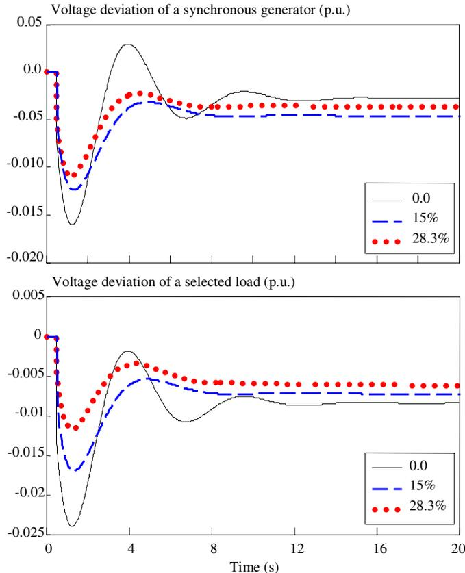
Fig. 9. Voltage deviation of one of the synchronous generators and a selected load as a result of switching a load of 10Mvar in the high-voltage network
