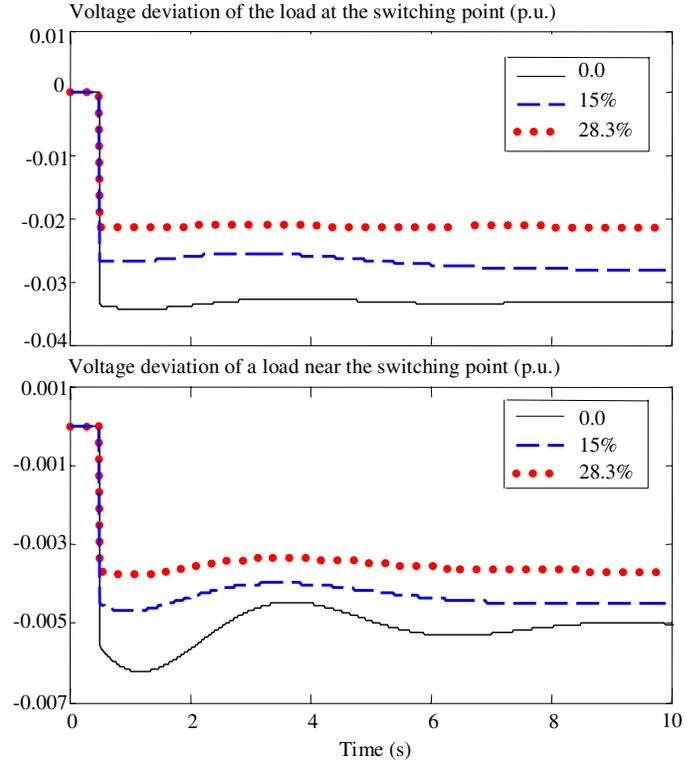
Fig. 10. Voltage deviation at two load terminals as a result of a switching a load of 1Mvar in the low-voltage network
