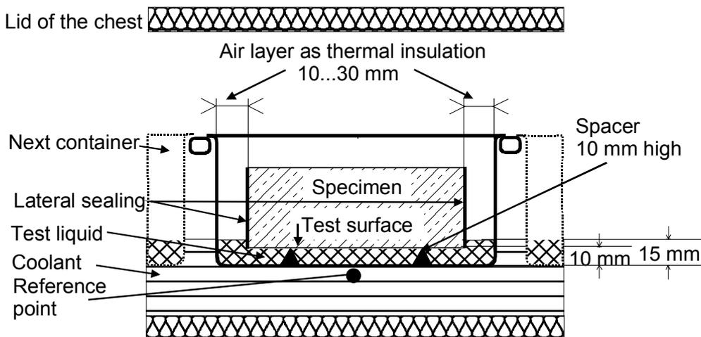
Fig. 2 Test container with specimen in the liquid cooling bath.
