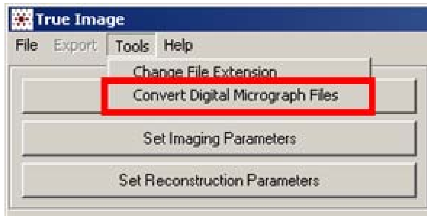
Figure 6.10: "tools"-options in TrueImage: changing of file extensions and converting of Digital Micrograph (.dm-files) into .dat-files is possible.
