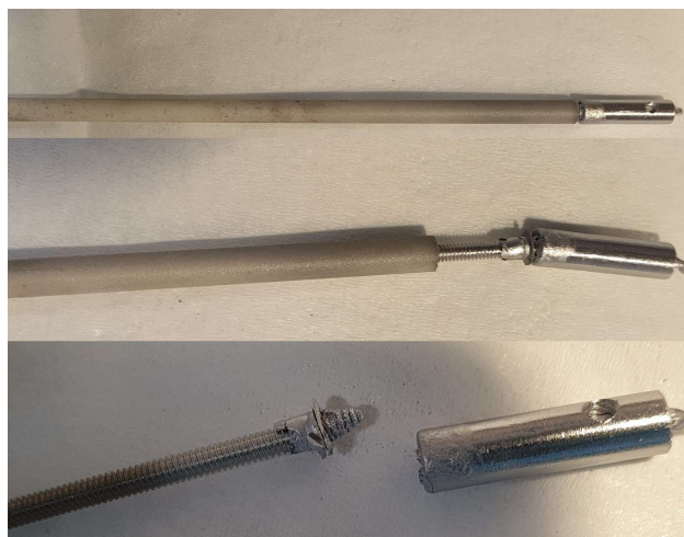
Fig. A.10.: The top image, shows the how the Rh rod should have been positioned. The middle picture shows the position of the Rh rod inside the evaporator and the ceramics were pulled back revealing some build up material. The bottom image shows the detached rod, that was barely holding on to the threading. The metallic material covered the whole steel threading and was even "flowing" inside the ceramics. A lot of material can be seen on the molybdenum rod holder as well.
