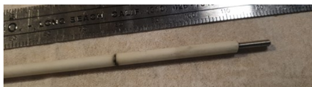
Fig. A.8.: Broken isolation, that went black as sparks could hit the underlying metal.
