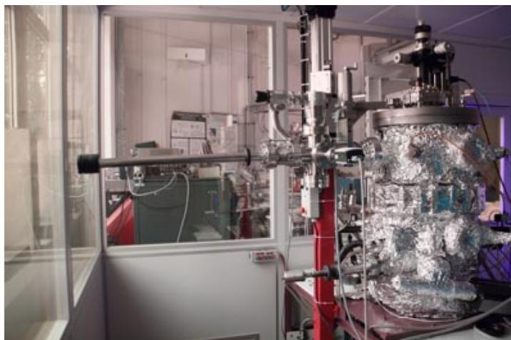
Figure 3.3: The electron beam evaporation setup that is used for thin film evaporation. The main chamber is on the right which is covered with aluminum film. On the left the transfer rod can be seen. (Uni Duisburg Essen / AG Farle)
