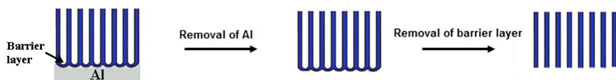
Figure 3.5. Represents the schematic of removal of remaining aluminum and barrier layer. During this process the pores diameter are widened.
