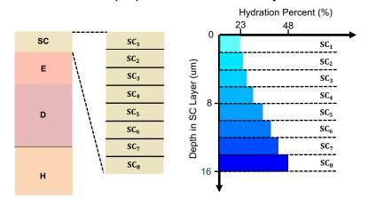
The dielectric properties of each sublayer of SC were calculated using Bruggeman's Effective Medium Theory [1] across the frequency range of 1–300 GHz.
