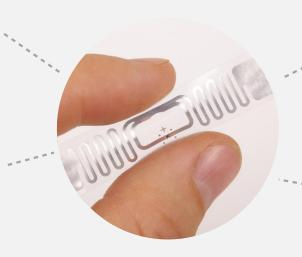
chipless RFID tags can be easily printed on different materials such as paper, polymer films, skin, glass, textiles and other objects in the world of products.
