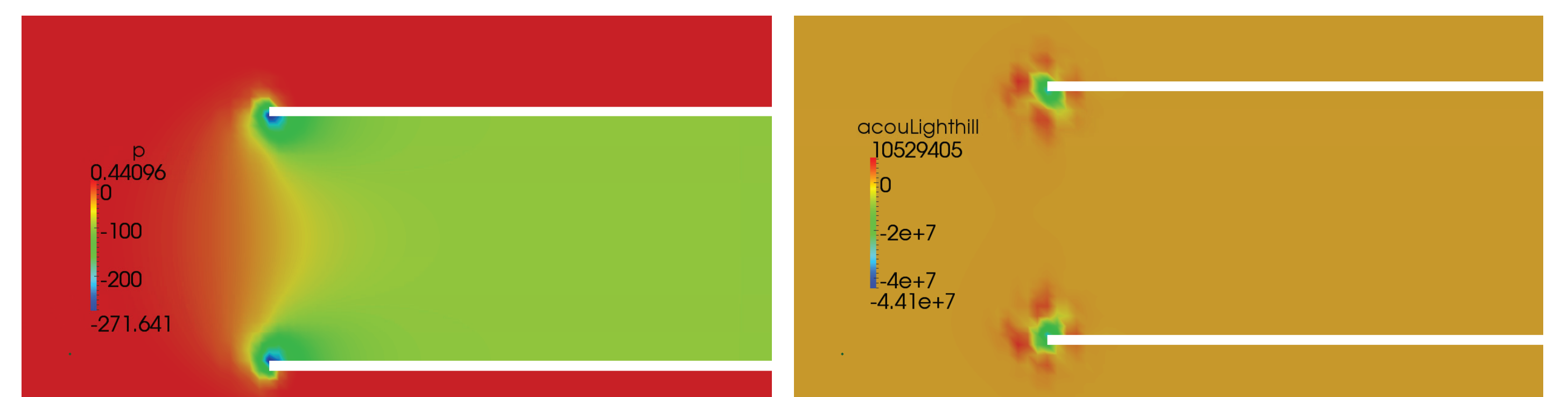
Fig.6: Computed pressure distribution and acoustic sources according to Lighthill at tube opening based on the incompressible, laminar steady state fluid simulation
