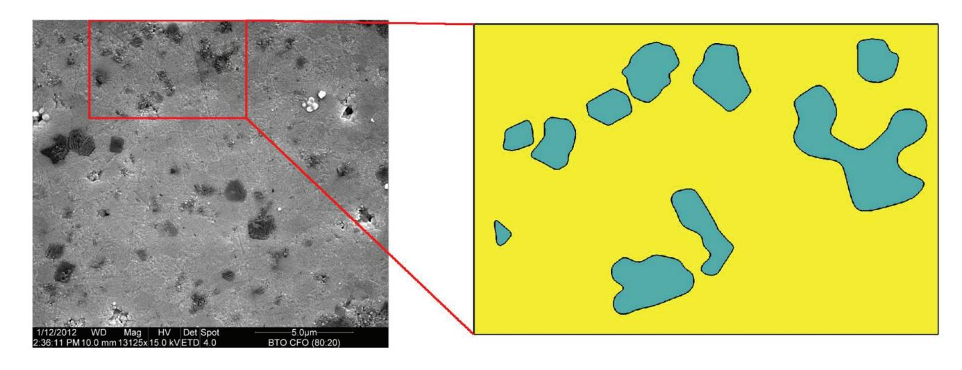
In order to analyze the ME coefficient we apply an external electric field  $\overline{E}_2$  in vertical direction. The resulting deformation of the piezoelectric matrix is transferred to the piezomagnetic particles so that a (strain-induced) magnetic induction is generated.
