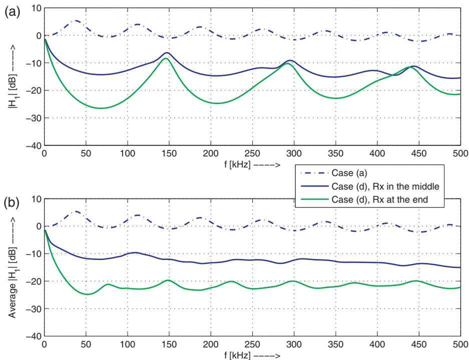
Fig. 4. Magnitude transfer function as function of frequency  $f$  for scenario (d) from Fig. 2 with different locations of the receiver (Rx). Curve for scenario (a) included as a reference. (a)  $|H_1|$  from (2), (b) average of  $|H_1|$  for 100 random line networks.
