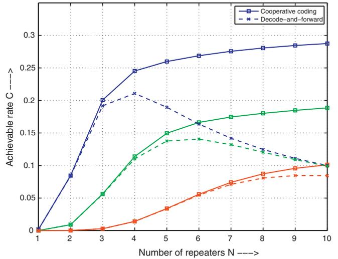
Fig. 8. Achievable rate for cooperative coding  $C_{\text{coop}}$  and decode-and-forward  $C_{\text{df}}$  as function of number of repeaters  $N$ . Link of 1 km and attenuation of {40, 60, 100} dB/km (curves from top to bottom).
