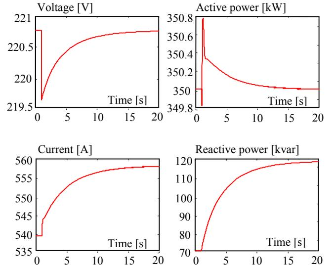
Fig. 5. Response of a selected fuel cell to load switching
