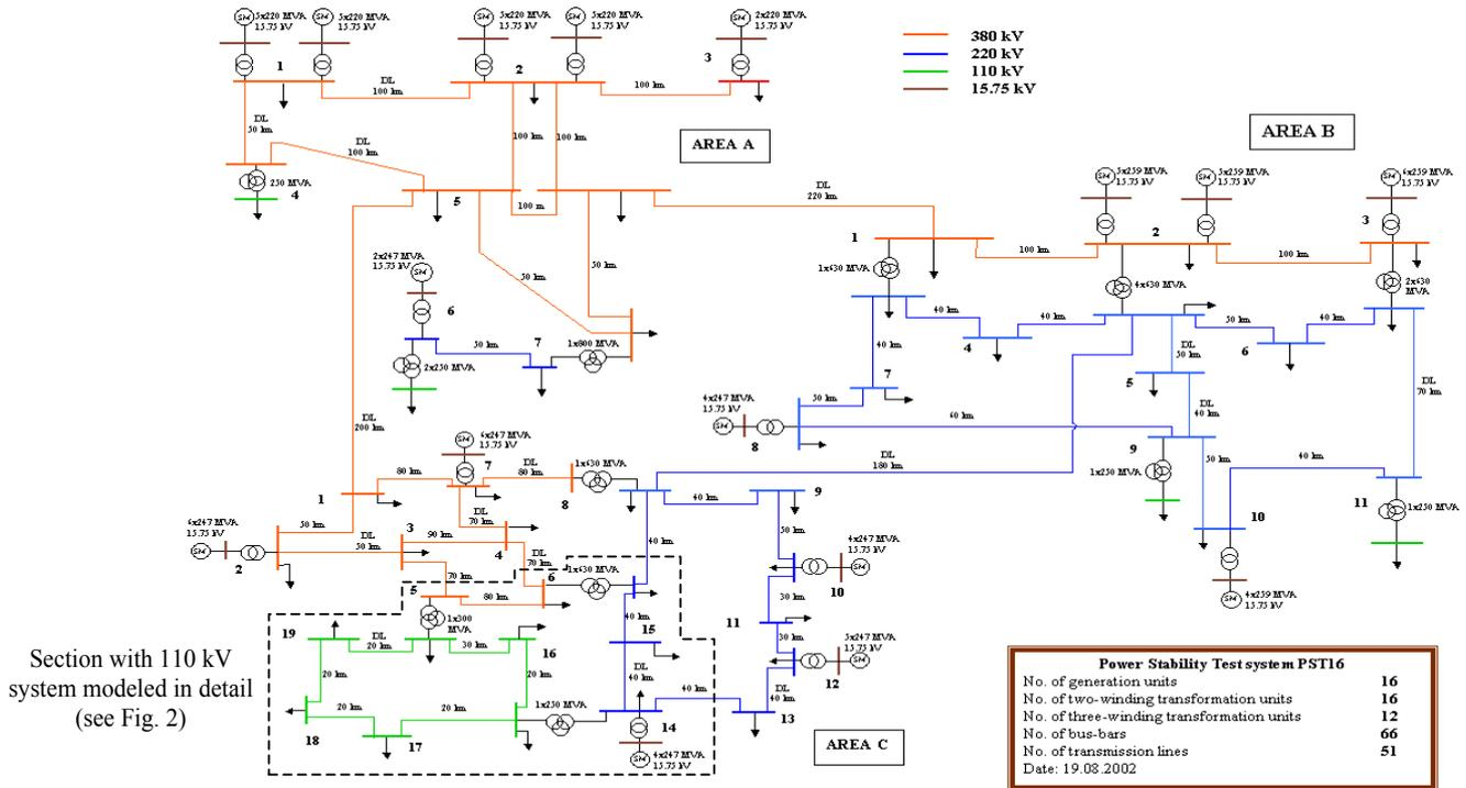
Fig. 1. Single line diagram of the PST16 network
