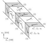
Co-existence of martensitic twins and ferromagnetic domains: experimental and schematic visualization of microstructure in MSMA. Variant volume fractions  $\xi_i$ , net magnetizations  $\eta_i$ , orientation of the magnetization directions  $\theta_i$ .
