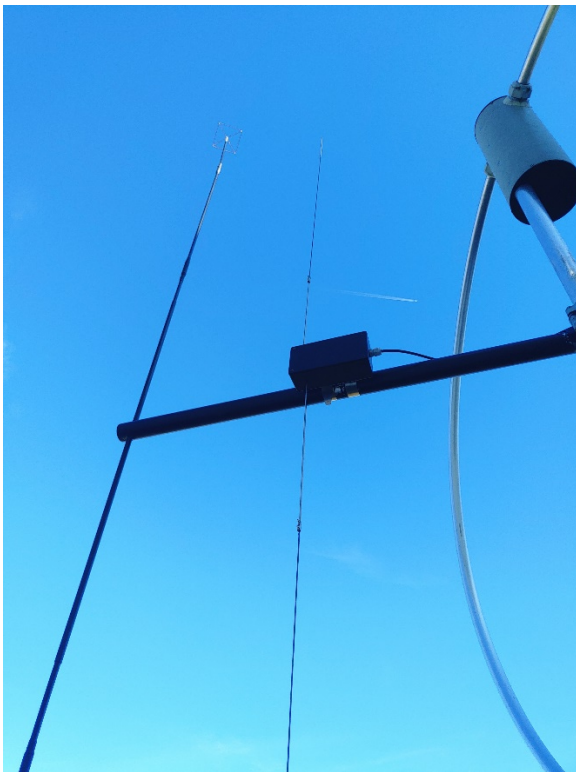
Figure 1: 2 x 5/8 \lambda (lambda) dipole for VHF between shortwave dipole and shortwave MagLoop
