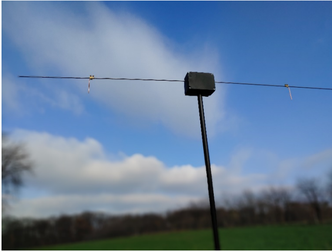
Figure 10 The antenna in portable operation in horizontal polarization on a GRP rod.
