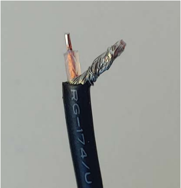
Figure 2 Test cable with open-circuit. The inner conductor and outer conductor are separated at the end and are approx. 6 mm long.
