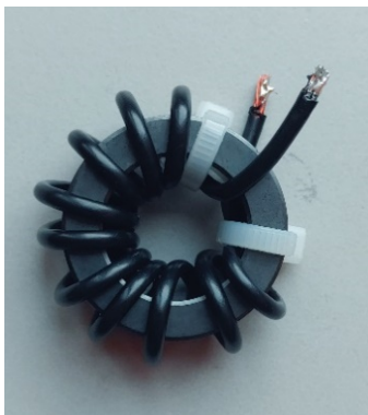
Figure 16 Current balun for the HF range made of 10 turns RG174 on FT 140-43.
