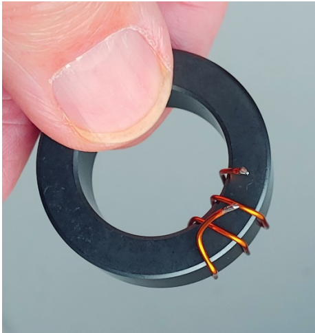
Figure 11 Coil with 3 turns on FT 140-43 ferrite core.
