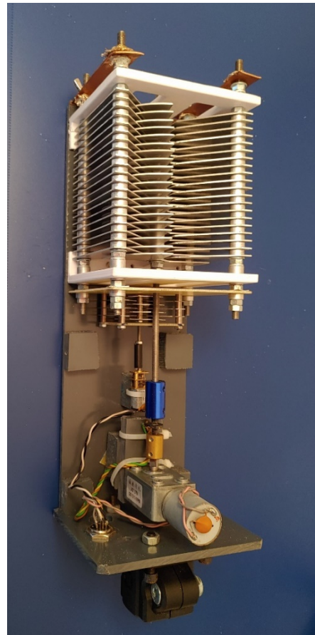
Figure 9 The variable capacitor (upper part) of the MLA with drive motors (below)
