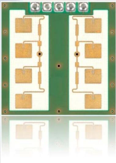
The task of the thesis is to build a Doppler Radar demonstrator using the IVS-465 module as the Radar sensor, realizing a mother board for the module and two audio filter / amplifier circuits and using a notebook computer to process the Doppler signals and display the measured target velocity.
