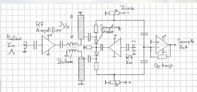
The thesis task is to design, build and test a sampler circuit for the frequency range of 1 to 4 GHz. The sampler is to use a pair of Schottky diodes in a bridge configuration employing a balanced injection of the sampling pulse and an unbalanced RF signal injection, realized as a printed circuit board (PCB). The sampler is to include a biasing
