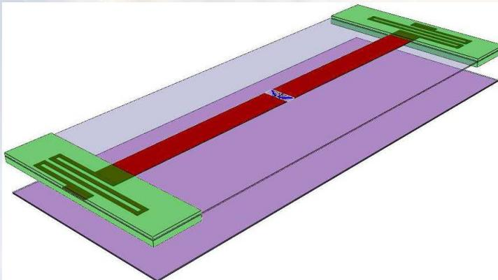
coil uses a metallic shielding plate of width and length as the meander dipole spaced some 10 mm below the dipole. For the dipole antenna in free space, it was found that the limited size of the shielding plate makes it act like a director in a Yagi antenna, directing radiation power away from the dipole in its direction. Nevertheless, with the dipole is loaded by an absorbing medium (the patient or a
