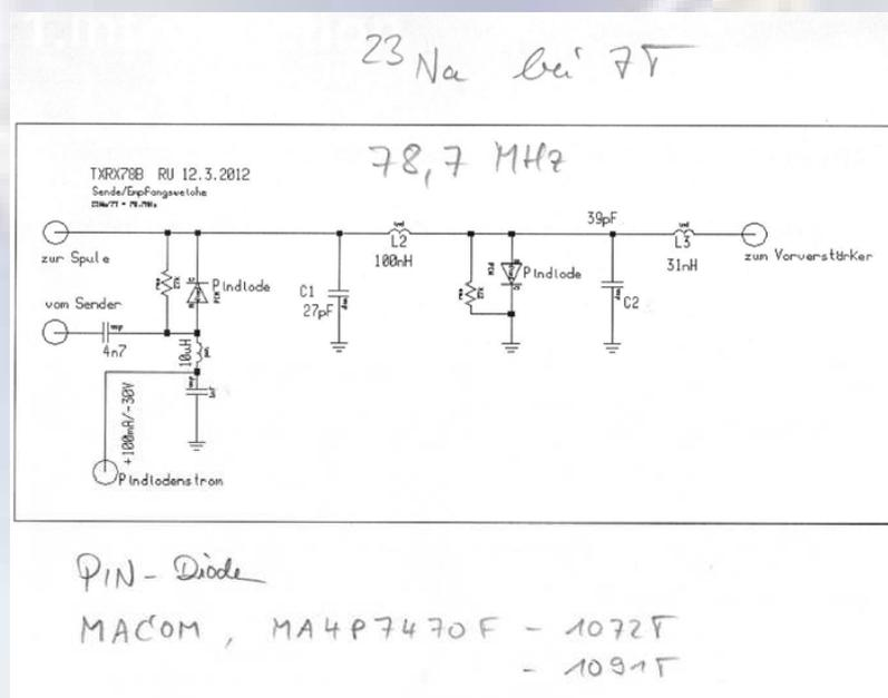
In order to allow the use of the coil in receive and transmit, a transmit/receive switch has to be inserted between the high-power transmitter and the receiver lownoise amplifier. A suitable switch design has been prepared as shown below, which employs PIN diodes as electronic switches which are embedded in a RF circuit. The diodes are biased in reverse (-30V) and forward (+100 mA) to act as open or closed switch.
