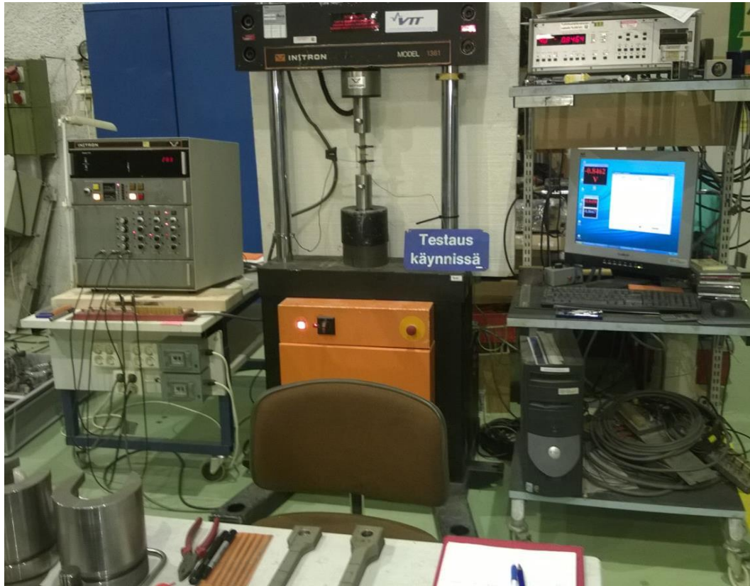
Fig. 3. The servo-mechanical test machine used for the relaxation tests.
