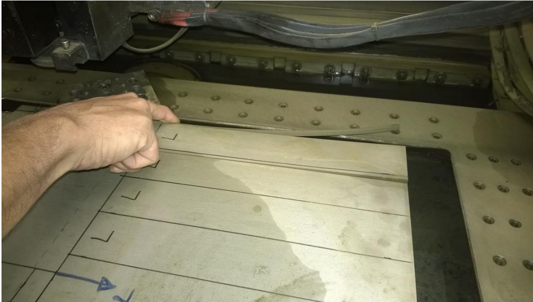
Fig. 2. Bending caused by residual stresses during wire erosion.
