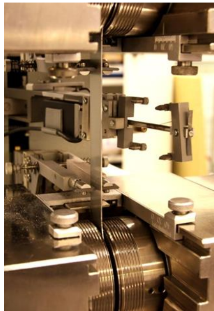
Figure 3. Hydraulic specimen grips and Zwick macro extensometer.
