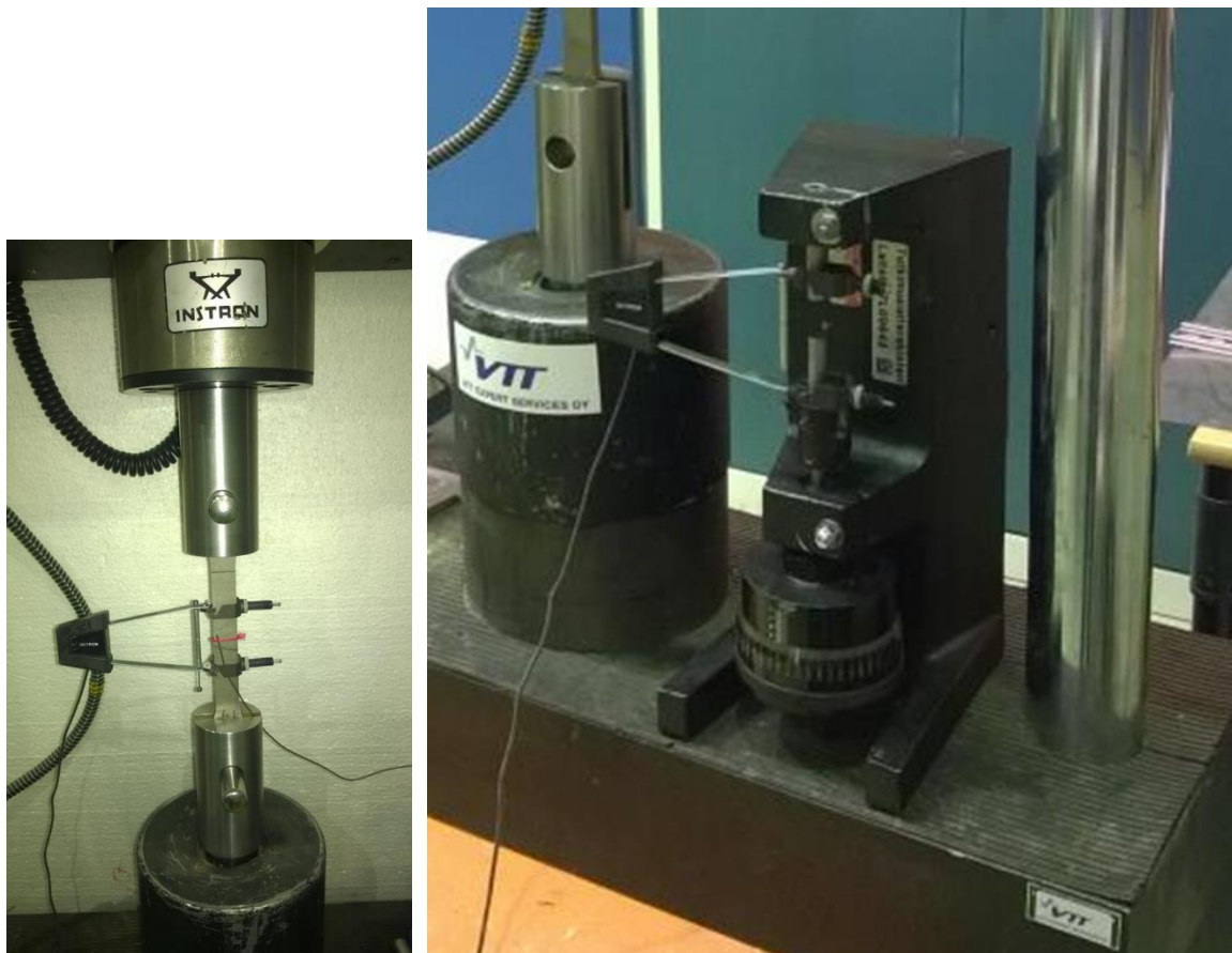
Fig. 4. The test specimen with a strain transducer and a thermocouple during the test (left) and the set-up used for the calibration of the strain transducer (right).
