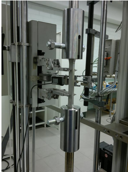
Figure 6. Short term creep test specimen in the pin-end grips.
