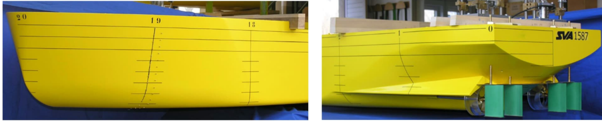
Figure 1. Inland waterway ship model, built at Schiffbauversuchsanstalt Potsdam (SVA), designed by DST.
