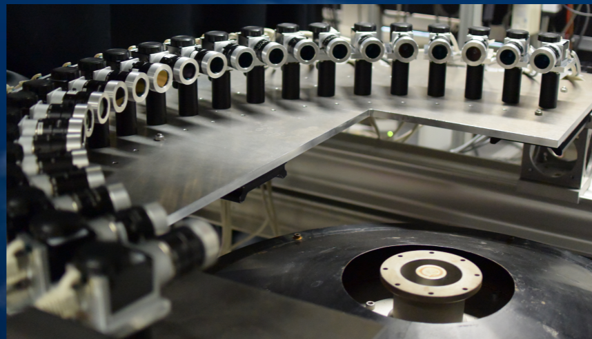
Image of the existing tomography setup around a burner.
