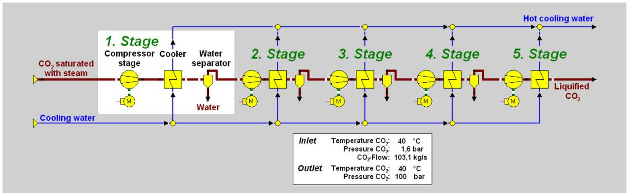
**Figure 3:** Supercritical liquefaction of the saturated CO<sub>2</sub> for a compressor with five stages
