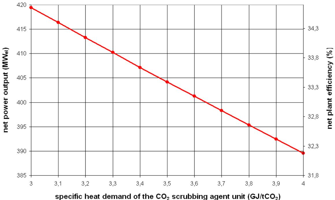
**Figure 5:** Net power output and net plant efficiency depending on the specific heat demand for the flue gas scrubber
