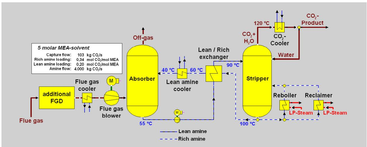
**Figure 2:** Model of the amine-based flue gas scrubber
