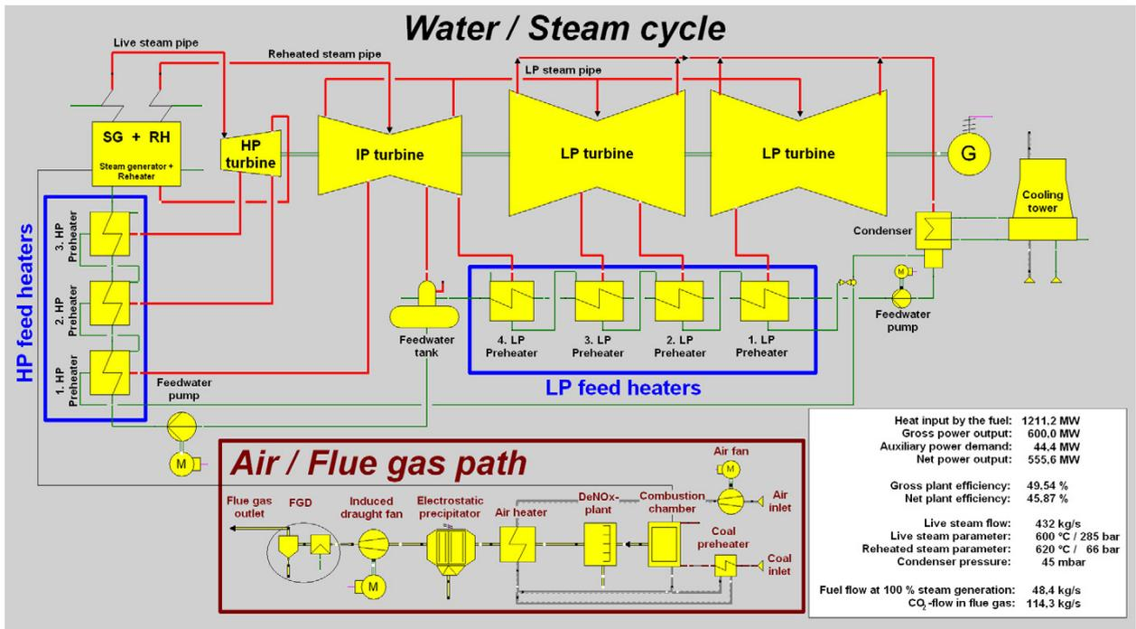
**Figure 1:** Process flow diagram of the coal-fired power plant in EBSILON® Professional
