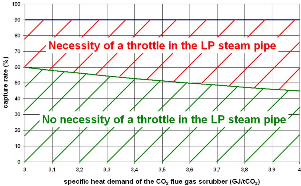
**Figure 4:** Capture rate of the power plant without and with installation of a throttle in the LP steam pipe depending on the specific heat demand of the flue gas scrubber by keeping a minimum pressure of 3,6 bar in the LP steam pipe
