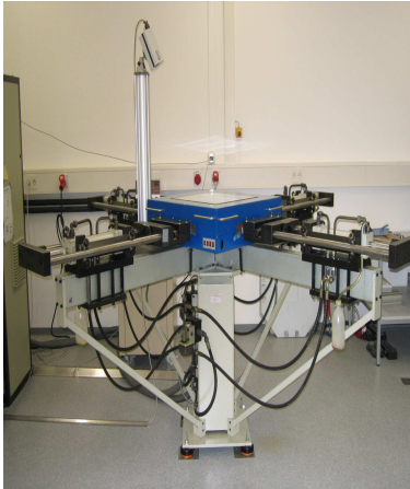
Figure 7.15: a) Machine for biaxial tension tests. b) Load-strain behavior of a PVC-Polyester composite.
