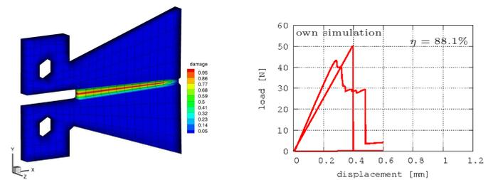
Woven fiber composite structure - distribution of damage:
