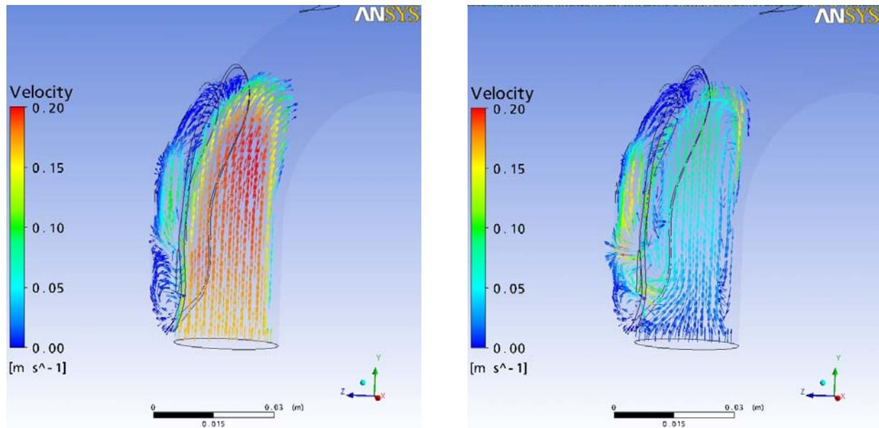
The experimental determination of the fluid velocity in the model ascending aorta is carried out using Particle Image Velocimetry (PIV). For the numerical simulation of the fluid flow the solver based on the Finite Volume Method implemented in the ANSYS CFX framework is used. Hereby both Newtonian and non-Newtonian fluid properties are applied. The non-Newtonian characteristic of the blood is modelled with the Ostwald–de Waele power law and Casson model.
