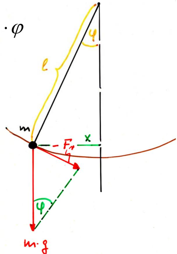
2. Newt. Axiom       $m\ddot{x} = ml\ddot{\varphi} = -mg\varphi$
