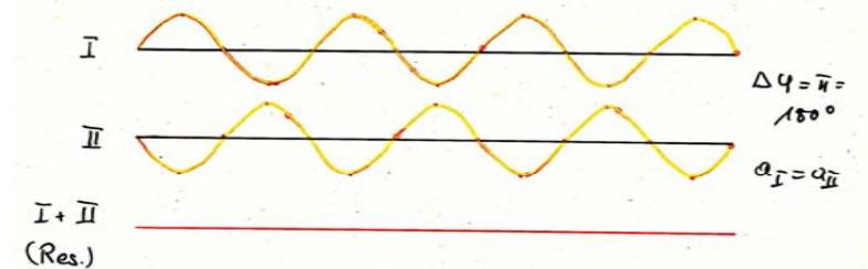
$$x(t) = x_I(t) + x_{II}(t) = a_I \sin(\omega t + \varphi_I) + a_{II} \sin(\omega t + \varphi_{II})$$
