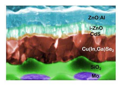
A solution to our world's increasing energy demand is right out there: the sun! Chalcopyrite solar cells, made mostly from Cu, In, Ga and Se, have the potential of contributing a significant share to the photovoltaic market. Addressing the limited supply of indium, which will restrain their production in the upper GW scale, we fabricate ultrathin and micrometer-sized absorbers. Losses emerging from the reduction of absorber material are tackled by optical concepts on the nano- and microscale.
