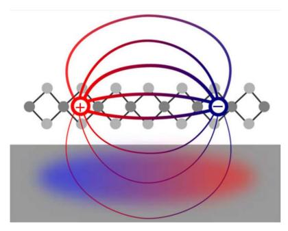
Layered semiconductors, like MoS2 or other transition-metal dichalcogenides (TMDC), exhibit particular opto-electronic properties due to their two-dimensional structure. Electronic states, like excitons, are predominantly confined to a single monolayer, but (in the case of multilayer or bulk samples) can also extend to neighbouring layers. Furthermore, they respond to charges and to dielectric polarizability in spatial vicinity, e.g. when a TMDC monolayer is deposited on a substrate.
