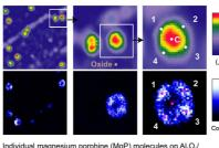
Individual magnesium porphine (MgP) molecules on Al<sub>2</sub>O<sub>3</sub>/ NIAI(110). V<sub>sus</sub> = 2.2V, I = 20pA. Scan size from left to right: 24nmx24nm, 6.8nmx6.8nm, 3.5nmx3.5nm. The individually adsorbed MgP molecules show a tunneling current induced photoepicing.
