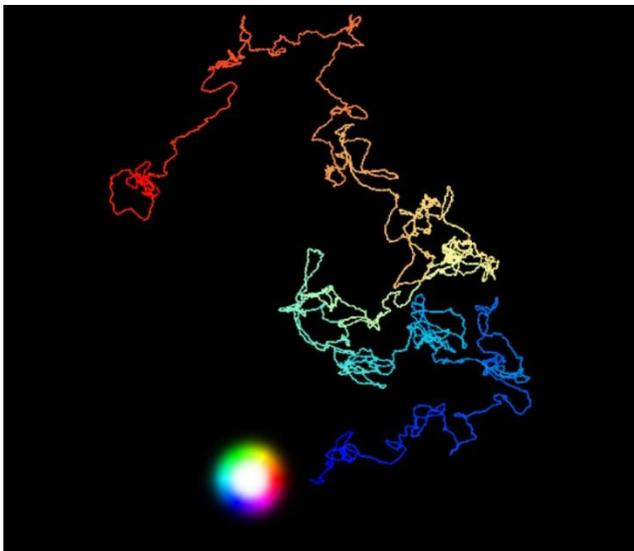
The dynamics of magnetic skyrmions are governed by the complex interplay between driving forces, thermal fluctuations and material disorder. This interplay leads to rich behavior, e.g. a creep motion that persists up to almost 100 m/s, which needs to be fully understood before skyrmions can be reliably used in technological applications like the racetrack memory [1].
