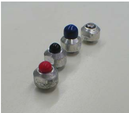
Figure 5. Different tips of the impulse hammer (used as contact device)
