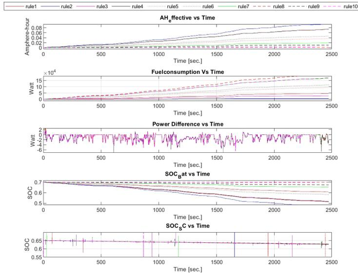
Fig. 5. Variation of powertrain parameters with rules for WLTP cycle
