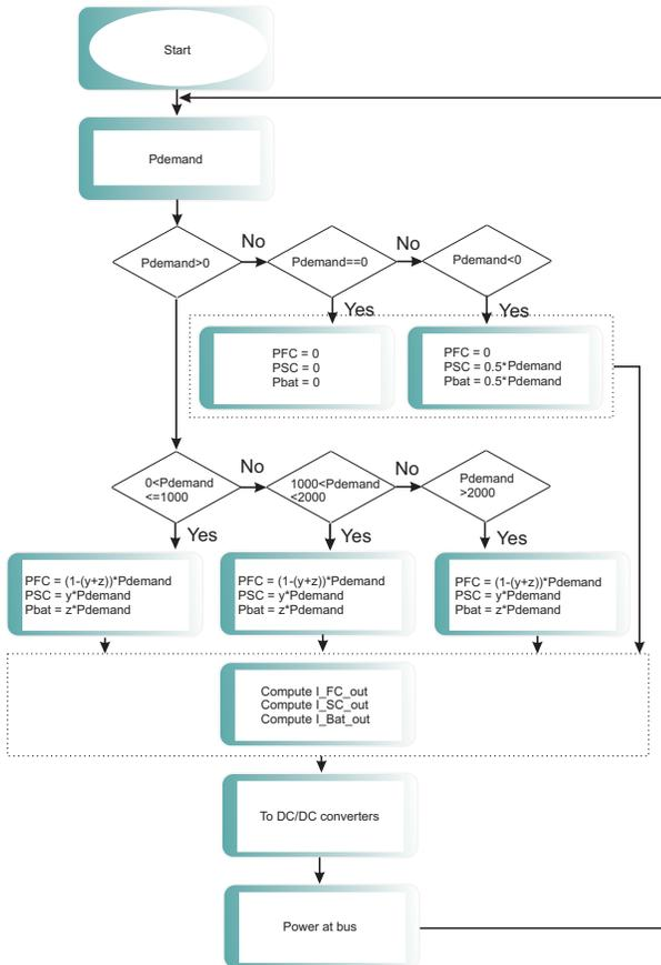
Fig. 2. Rule-based logic
