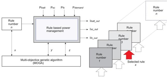
Fig. 1. Selection of optimal rule and powersplit
