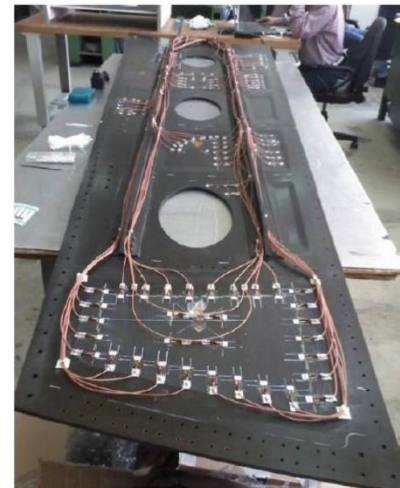
Sensor placement on the wing box [Marzani et al., 2019]
