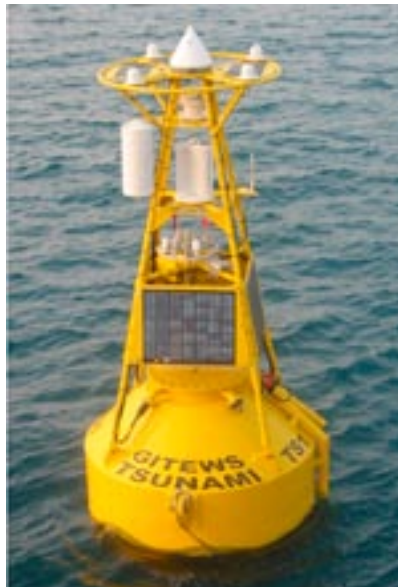
Tsunami buoys are being used for measuring changes in the ocean waves. Early warning systems are one example for research collaboration on a global level.
