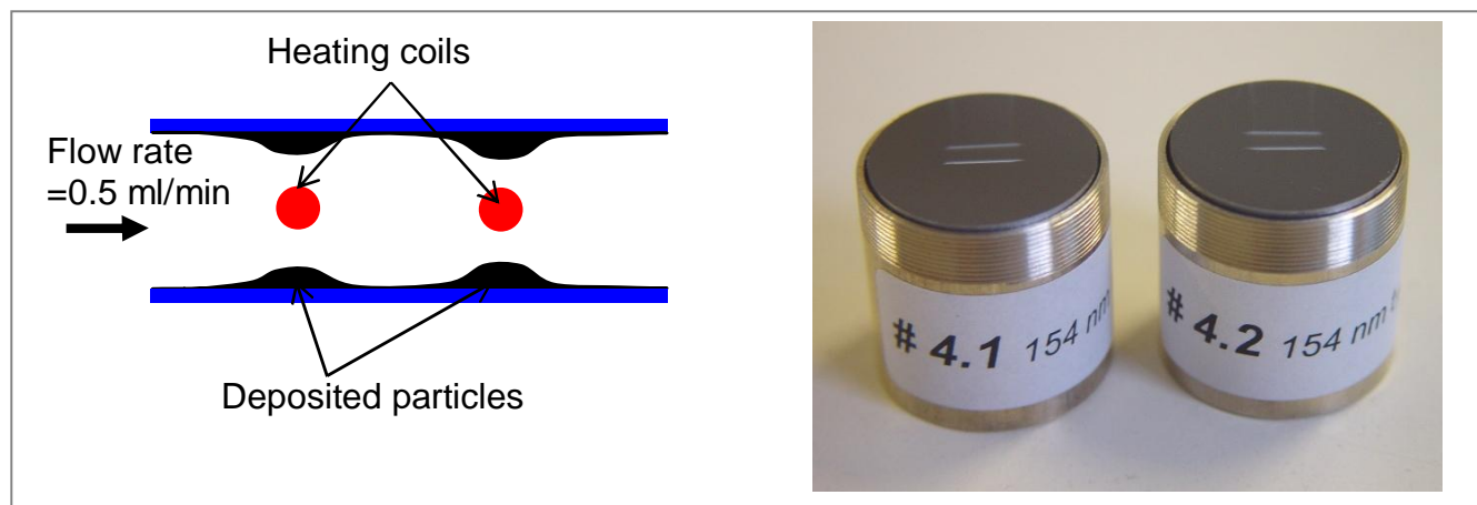
Fig. 3.1 2D Schematic of the TP1 showing its deposition characteristics and image of TP1 substrates after sampling
