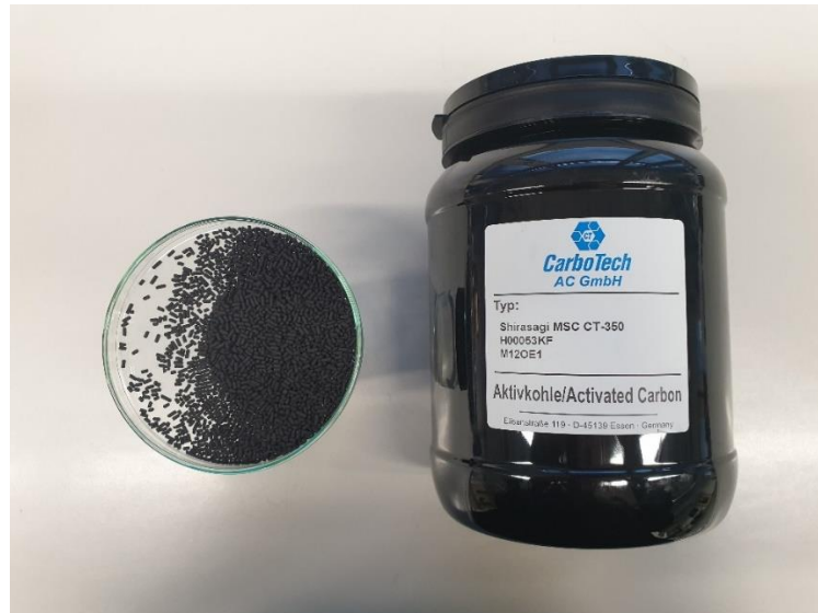
Fig. 4.1-2 Adsorbent Shirasagi MSC CT-350
