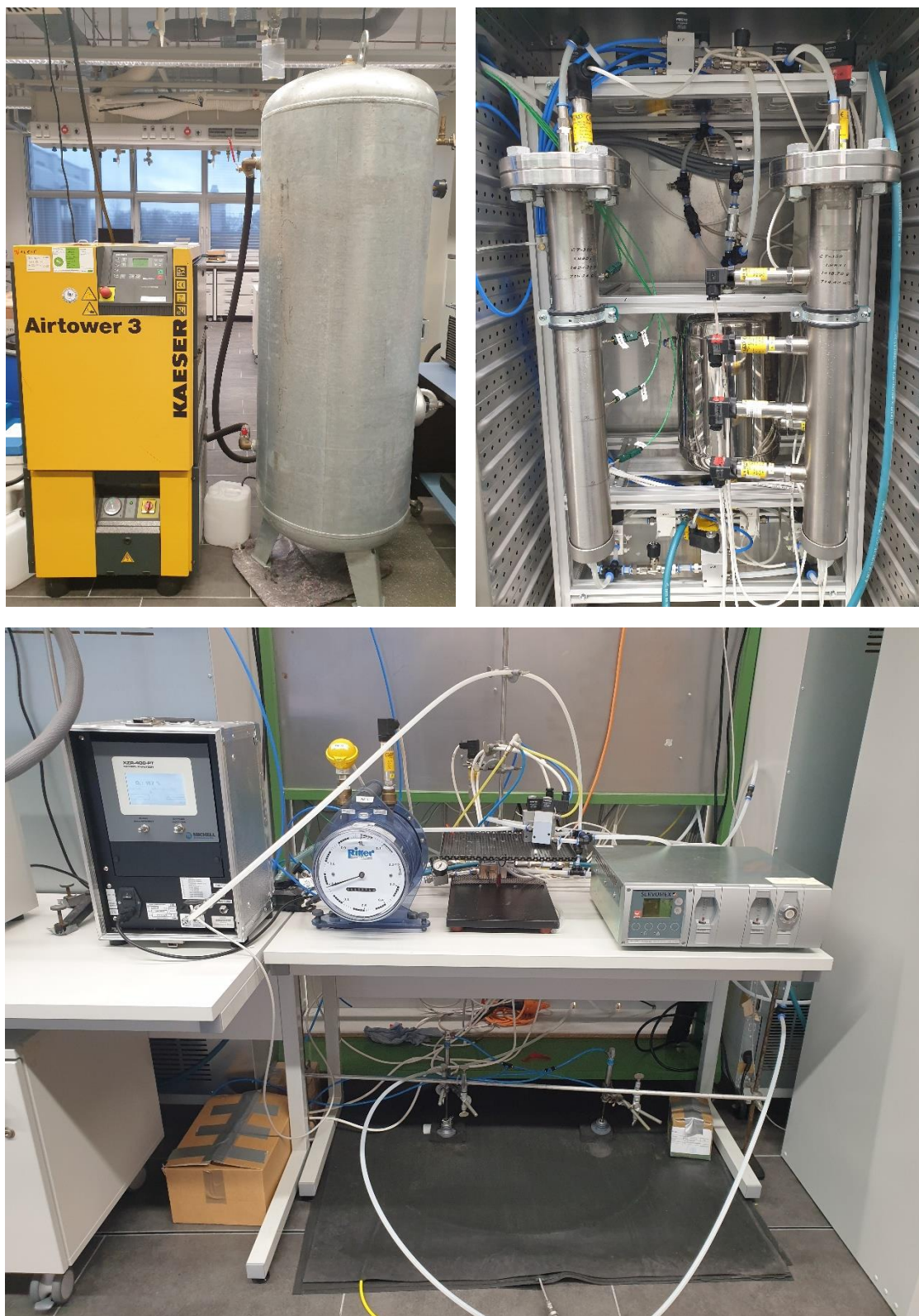
Fig. 4.2-2 (top left) the feed gas preparation and pre-treatment section; (top right) the twin-bed PSA plant section; (bottom) the product and tail gas analytics section
