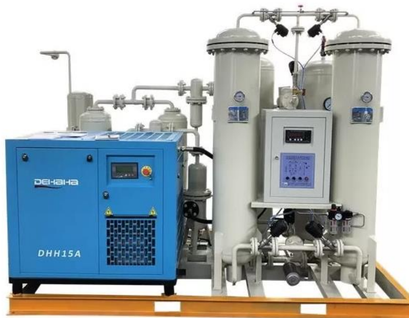
Fig. 1.1-5 Industrial-scale twin-bed N 2 -PSA skid [23]
