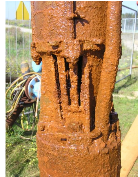
Ochreous deposits on pump. Source: B. Dericks
