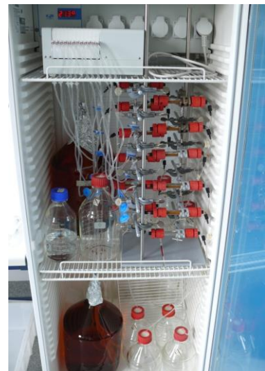
Test of survival of target organisms in ochre over time under flow through conditions
