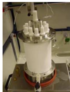
Annular reactor for investigation of the influence of water temperature on incorporation, persistence and survival of hygienically relevant bacteria in drinking water biofilms.
